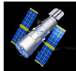
To improve the views of space, astronomers are able to access images from a telescope in space. Free from the interferences of weather, clouds humidity and even high winds, the **Hubble Space Telescope**, launched in 1990, orbits 373 miles above the Earth, collecting images of extremely distant objects. It is a cylindrical reflecting telescope, 42.6 ft long and 14 ft in diameter. It is **modular** (parts can be removed and replaced) and is serviced by shuttle astronauts.
