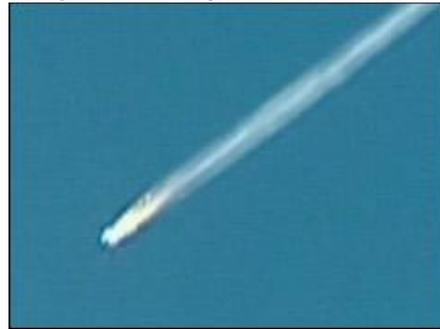
The loss of some insulating panels on the Shuttle Columbia during launch was the cause of overheating and eventual disaster (explosion of the shuttle) during its re-entry, after a successful mission in space. 7 astronauts lost their lives
