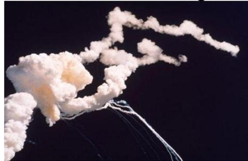
A faulty O-ring on the booster rocket, carrying the Shuttle Challenger, caused the explosion during takeoff which took the lives of 7 astronauts.
