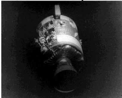
An explosion on the exterior of the Apollo 13 capsule cut short the mission to the moon. The 3 astronauts aboard the capsule were able to use the LEM (Lunar Excursion Module) for life support until their successful re-entry.
