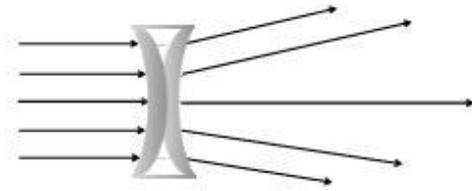
A **double concave lens** is thinner and flatter in the middle than the edges. Light passing through the thicker more curved areas of the lens will bend more than light passing through the thinner areas, causing the light to spread out or **diverge**.
