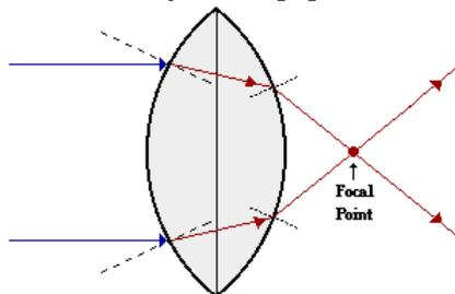
Incident rays which travel parallel to the principal axis will refract through the lens and converge to a point.
