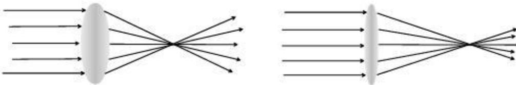
However, light from the left portion of the object is directed to the right and the light from the top is directed to the bottom. This **inverts** the image. Overhead projectors and film projectors do this.
