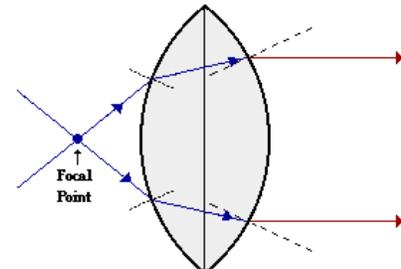
Incident rays which travel through the focal point will refract through the lens and travel parallel to the principal axis.
