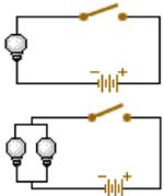
A **series circuit** provides only one path for the current to flow,
