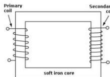
A **step-down transformer** reduces voltage.
