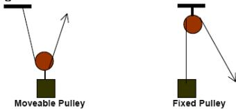
A complex combination of fixed and movable pulleys is called a **block and tackle**.
